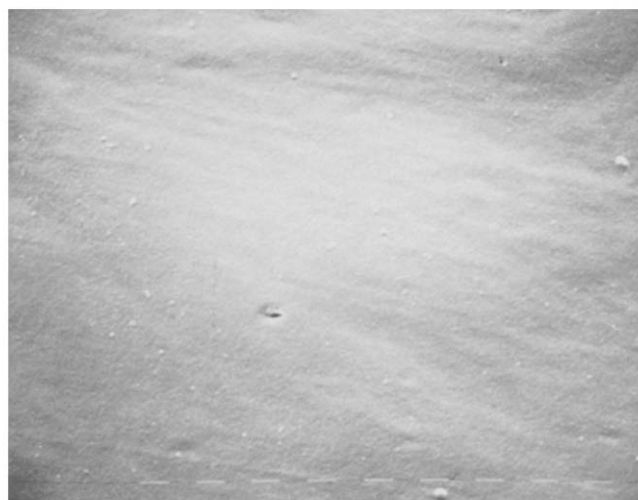
Figure 2 SEM micrographs of etched surfaces of iPP (n-heptane, 20 min) magnification 3600 \times
